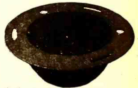
The Flux valve—heart of the Gyrosyn Compass.
