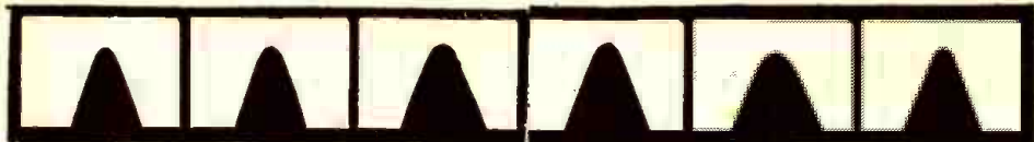
The various forms into which different types of needles wear, as seen in micro-photographs.
